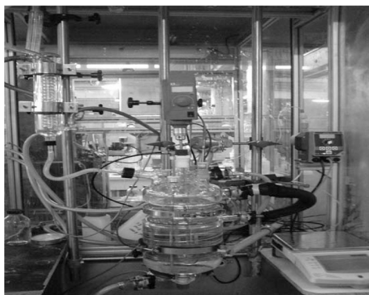
Figure 1. Experimental System (Calorimeter Reactor)
